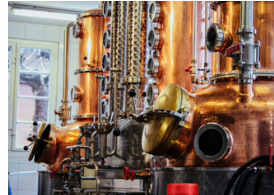
FASSBIND USES A HYBRID OF A POT STILL AND COLUMN STILL. A CATALYTIC CONVERTER IS INTEGRATED IN THE COLUMN STILL, WHICH IS VERY IMPORTANT FOR THE DISTILLATION AND CONCENTRATION OF FRUITS. THE TWO POTS FOR THE MASH HAVE A CAPACITY OF 350L EACH.
