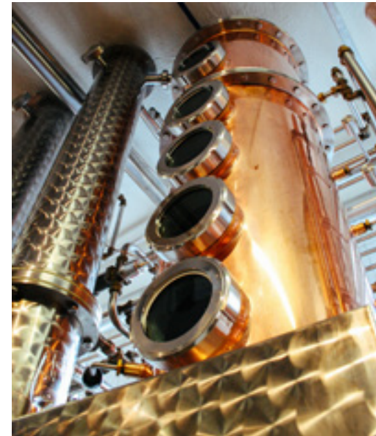
FASSBIND USES A HYBRID OF A POT STILL AND COLUMN STILL. A CATALYTIC CONVERTER IS INTEGRATED IN THE COLUMN STILL, WHICH IS VERY IMPORTANT FOR THE DISTILLATION AND CONCENTRATION OF FRUITS. THE TWO POTS FOR THE MASH HAVE A CAPACITY OF 350L EACH.
